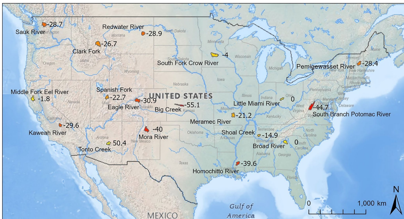
FIGURE 6 | Relative bias (%) in US Geological Survey (USGS) regional regression equations results in 18 test watersheds. Peak discharges at the 100-year (1% annual exceedance probability) scale are being underpredicted by regional regression equations (StreamStats) in most of the analyzed watersheds. [Color figure can be viewed at wileyonlinelibrary.com ]
