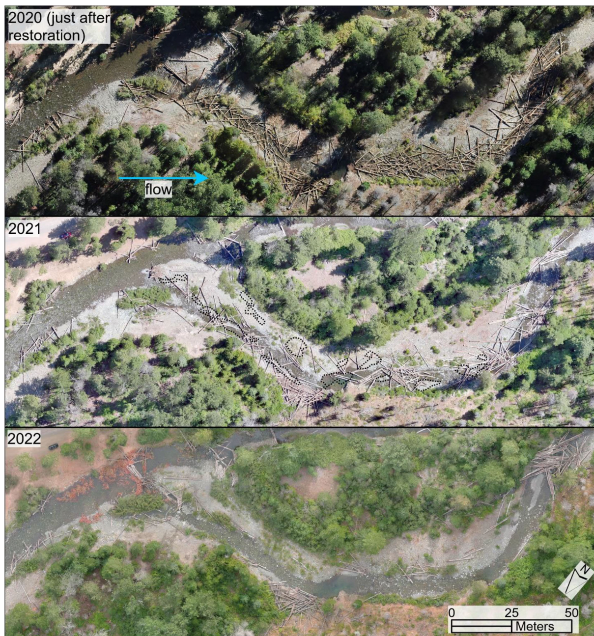
FIGURE 2 Repeat, orthorectified, georeferenced aerial photo mosaics showing the post-restoration wood assemblage along the North Fork Teanaway and its evolution over 2 years. Dotted black lines outline where fine sediment aggraded during 2020–2021. Credit Dan Scott. [Color figure can be viewed at wileyonlinelibrary.com ]
