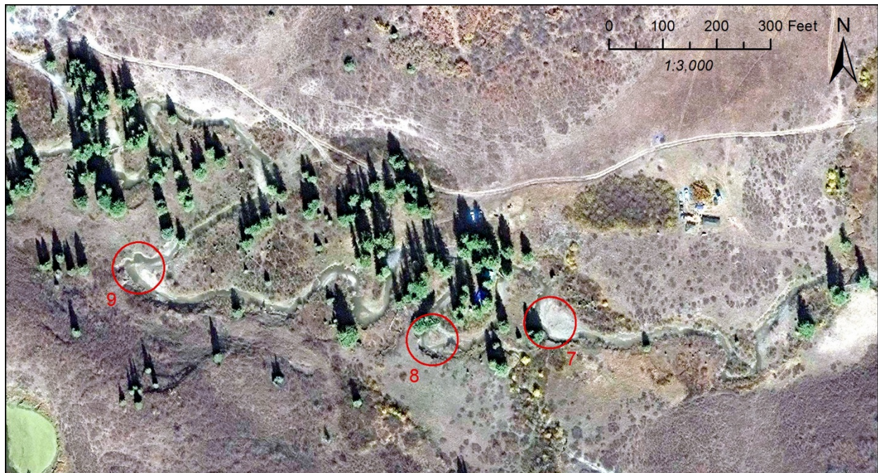
Figure 4: Aerial image detail of upstream portion of reach C (10/13/2016). Note the shadows and limited shading by tree canopy. The red numbered circles indicate streambank erosion locations of possible concern, with the numbers indicating the figures. Flow direction is from right to left.
