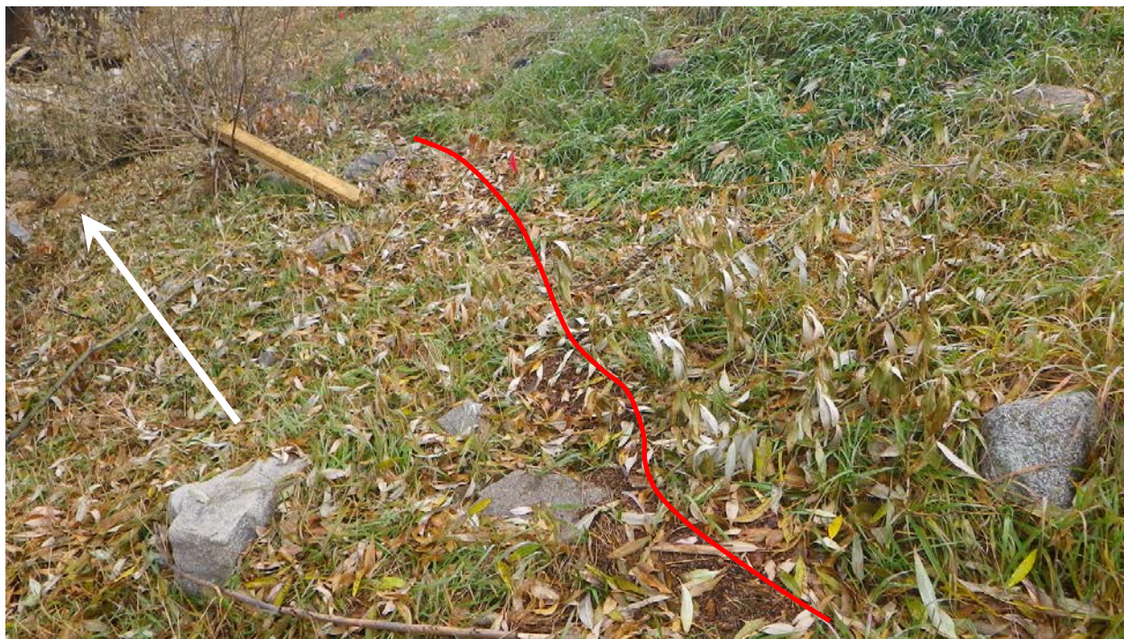
Figure 4: Series of high water marks, providing a peak water surface profile (James Creek).
