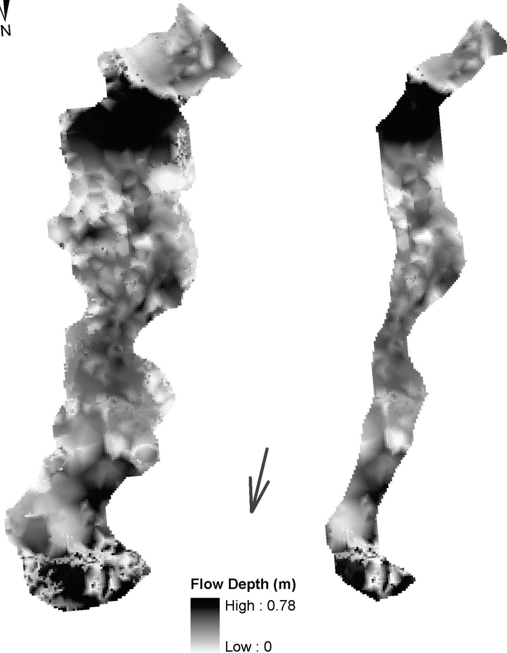
Figure D-11: Depth variability for mid flow, reach ESL-4 (7/14/2008).
