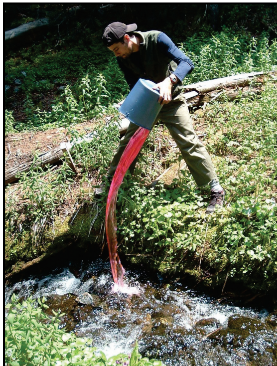
Figure 3-7: Rhodamine WT dye injection by field assistant Mark Hussey.
