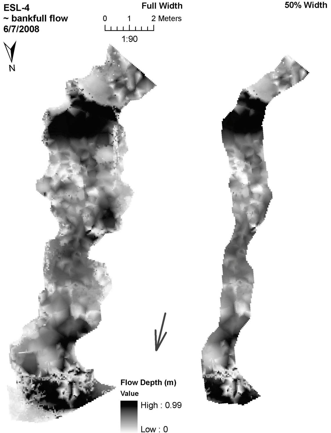
Figure D-10: Depth variability for ~bankfull flow, reach ESL-4 (6/7/2008).
