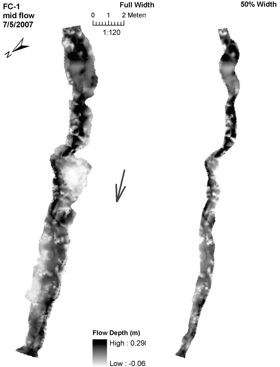
Figure D-27: Depth variability for mid flow, reach FC-1 (7/5/2007).
