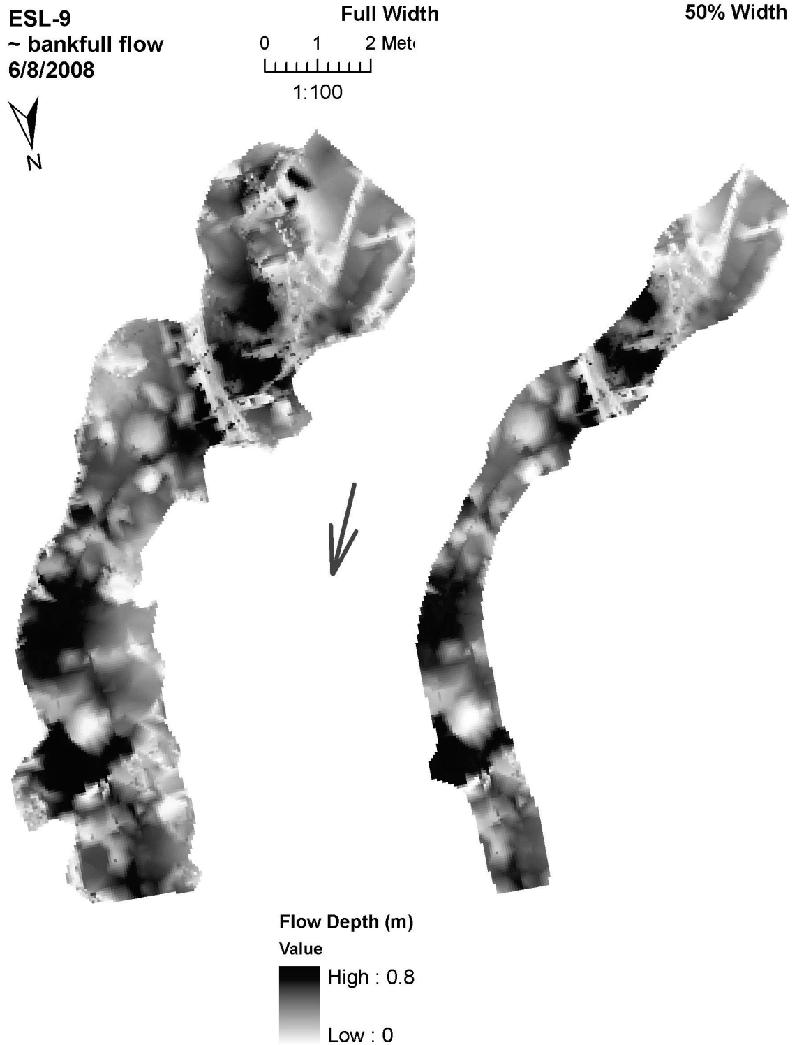
Figure D-25: Depth variability for ~bankfull flow, reach ESL-9 (6/8/2008).
