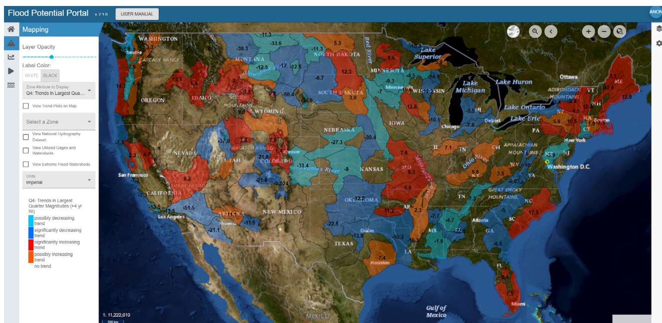
FIGURE 4 Significant and possible trends in flood magnitudes of the largest quarter (Q4) of annual peak discharges for streamgages within each flood potential zone, as viewed from within the Flood Potential Portal. Reds indicate observed increasing trends while blues indicate decreasing trends. Regions with the most consistent increasing trends in large floods include New England, the Interior Highlands, and the central portion of the Rocky Mountains. [Color figure can be viewed at wileyonlinelibrary.com ]
